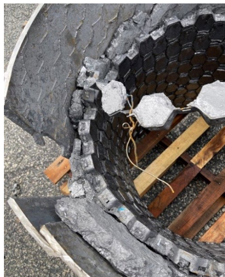
Left/Middle: A Reactor cyclone dipleg that required replacement within 3 years of operation due to bypassed refractory lining. Right: Carburized steel shell of at least 6mm after prolonged exposure to bypass.
