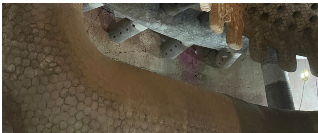
Thick layers of catalyst dust can be found in the regenerator, non-coking environments.
