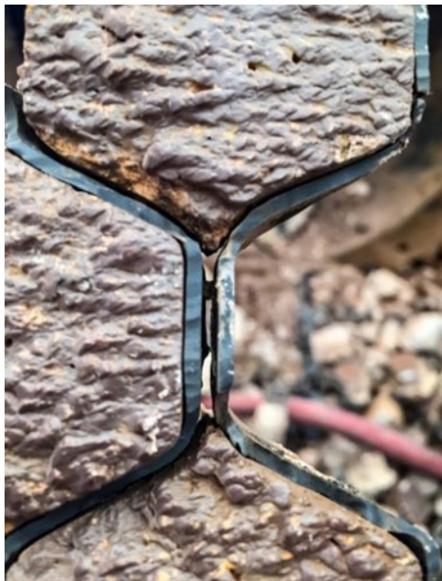
Inherent in its design, closed cell systems allow for pathways that reach behind the lining.
