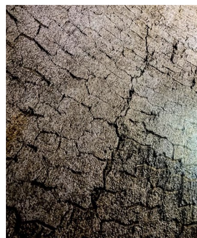
Runaway cracking in refractory.
