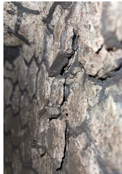
Biscuiting & Hex Spalling
