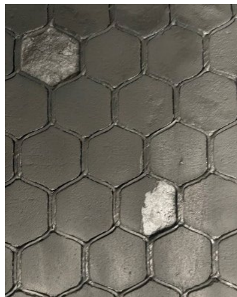
Refractory after coke absorption.
