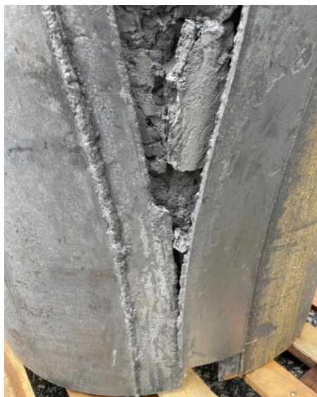
Left/Middle: A Reactor cyclone dipleg that required replacement within 3 years of operation due to bypassed refractory lining. Right: Carburized steel shell of at least 6mm after prolonged exposure to bypass.
