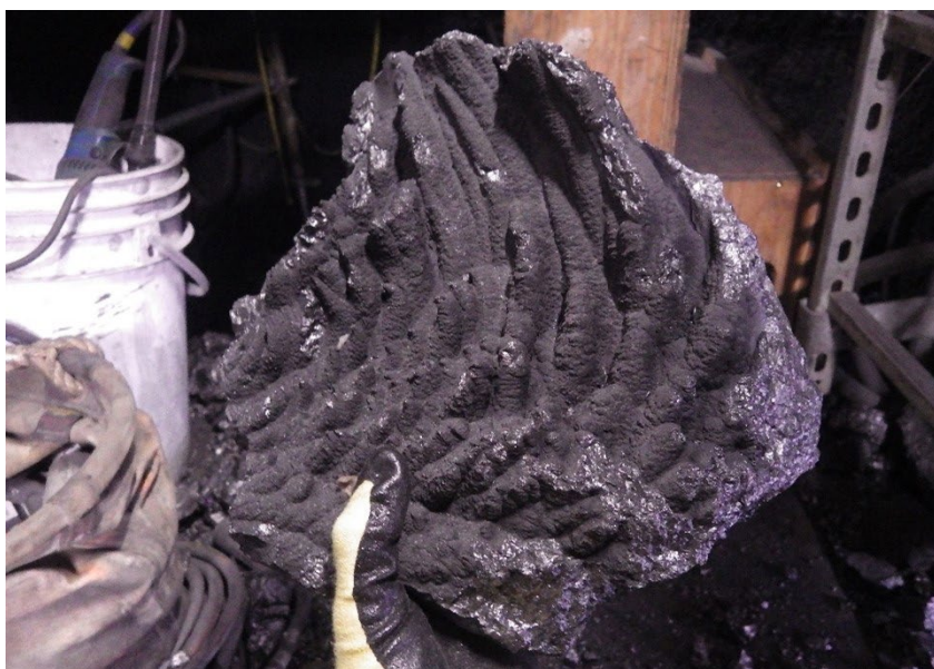
An example of built-up cokes formation.
