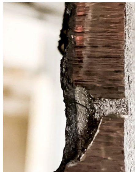
Left/Middle: A Reactor cyclone dipleg that required replacement within 3 years of operation due to bypassed refractory lining. Right: Carburized steel shell of at least 6mm after prolonged exposure to bypass.
